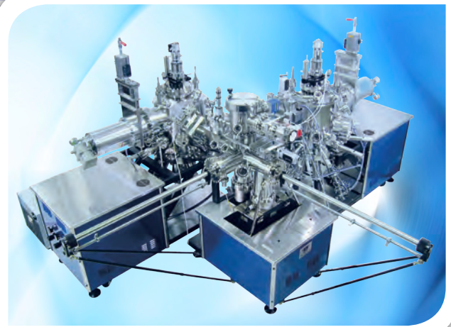
Multiple Material Nitride & Oxide MBE Configuration
